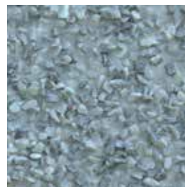
M: Medium Gradering: 3-5 mm
